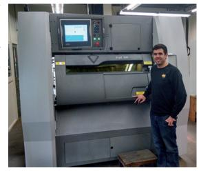
and implement additive manufacturing technology into their businesses, helping to reduce overall costs while bringing new products to market. An excellent example of this is their recent installation of a 3D Systems ProX 300 Direct Metal Sintering (DMS) printer at Mohawk Manufacturing in Middletown, Connecticut.
